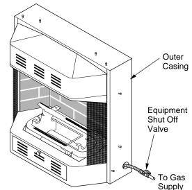
Figure 22 - Routing Flexible Gas Line
